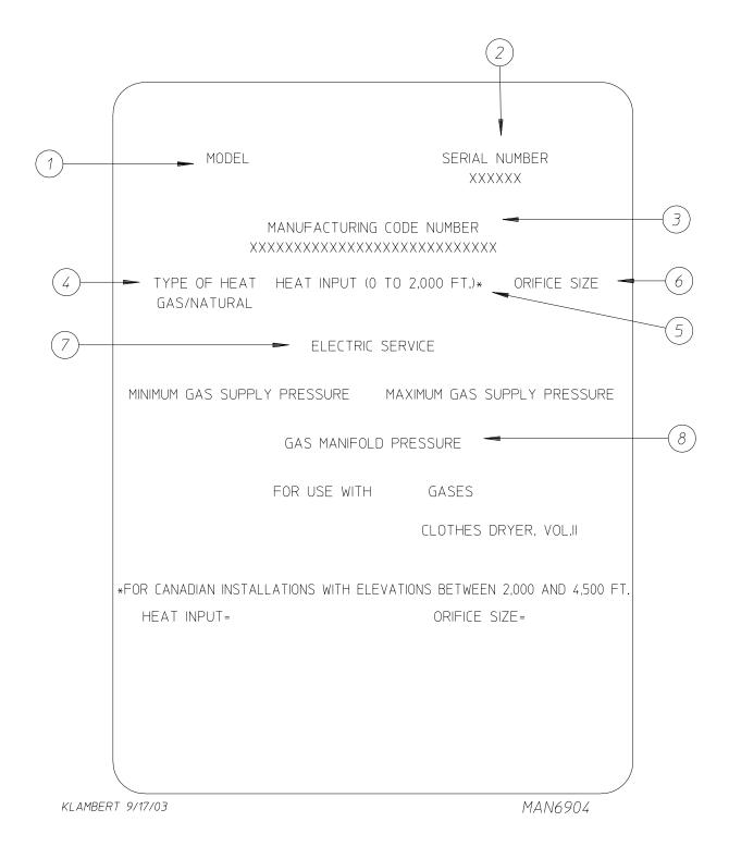
When contacting **American Dryer Corporation**, certain information is required to ensure proper service/parts information from **ADC**. This information is on the data label affixed to the left side panel area behind the top control (access) door. When contacting **ADC**, please have the **model number** and **serial number** available.
